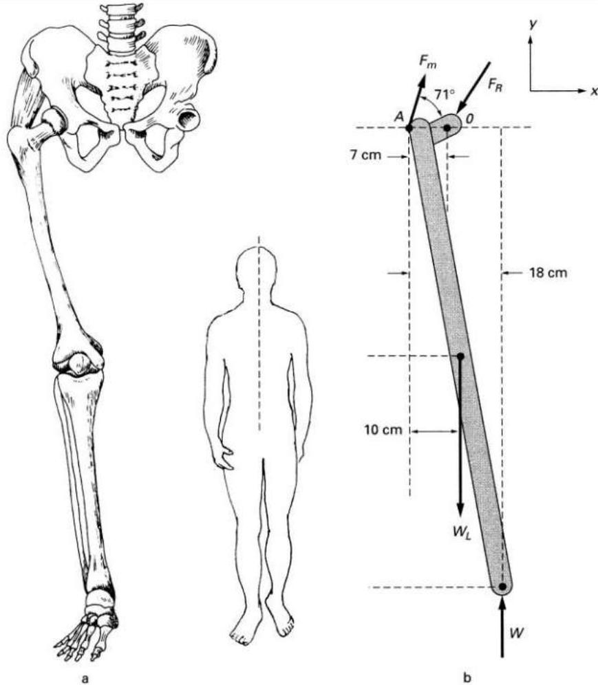
We will now calculate the magnitude of the muscle force  $F_m$  and the force  $F_R$  at the hip joint when the person is standing erect on one foot as in a slow walk,
